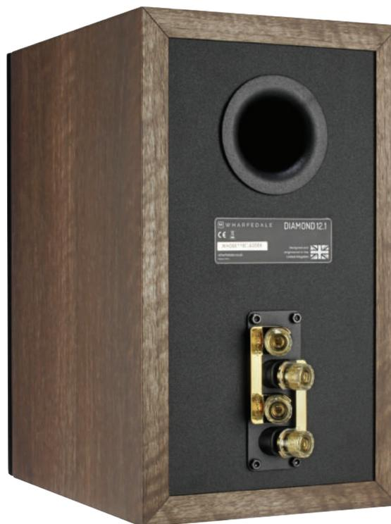
***The rear port has been optimised to work in unison with the drive units to assist low-end response. Two sets of terminals allow for optional bi-wiring with metal links provided for single wire connection.***
